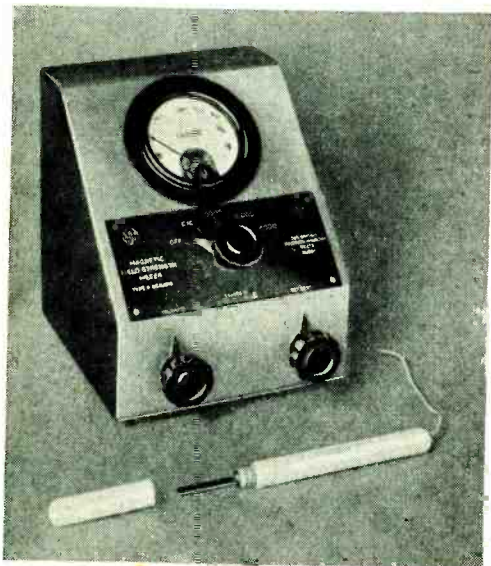
B.T.H. gauss meter, Type G, and (below) close-up of the probe, which is protected by a non-magnetic sheath.
